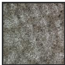
QUENCHING + TEMPERED AT 500°C
